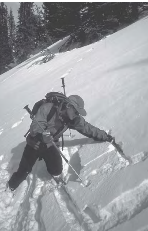
Photo 4-5. A quick test of surface layers: cut out a small block and tug on it.
