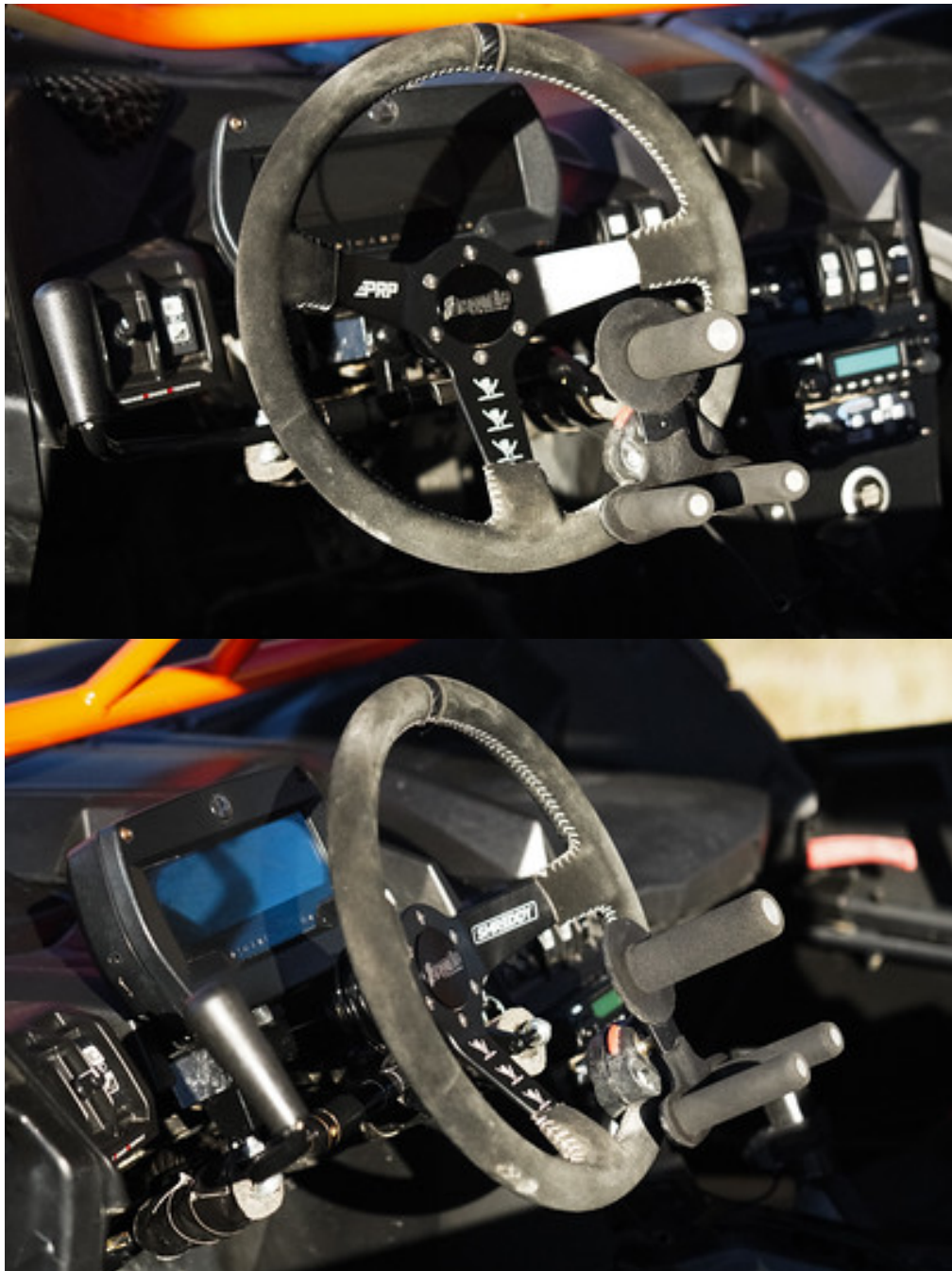
Figure 5: Can-Am UTV After-Market Hand Control Modifications for Adaptive Riders, captured by Brent Jacoby
